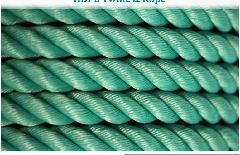
HDPE Twine & Rope: Our HDPE ropes are made of complete virgin, high density polyethylene. These ropes are "z" twist, medium laid, 3 stand ropes. We are prime manufacturer of an exclusive assortment of HDPE Ropes in Bangladesh. The excellent strength and flexibility possessed by our ropes make them widely demanded across various parts of Bangladesh. These precisionengineered ropes feature optimum abrasion resistance & improved durability and thus, of high utility for the market.
